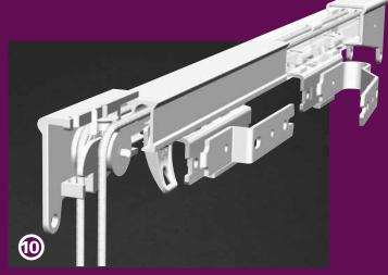
By pulling the cord through the big gap of the pulley, it will hang straight down the curtain and a good operation is guaranteed.
